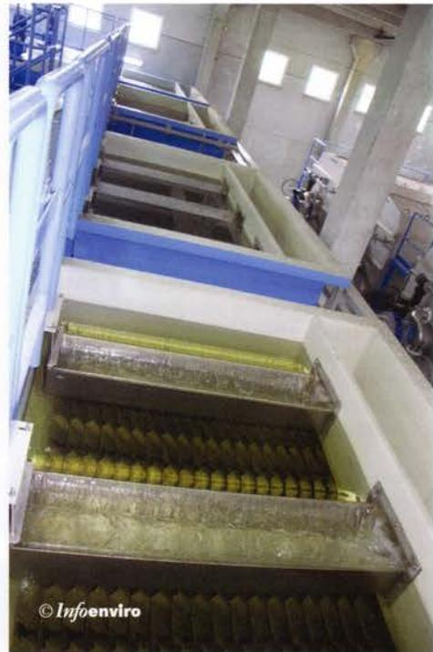
*Actiflo™ is a patented system based on chemical precipitation and lamellae plate settling combined with a new technology involving flocculation with micro-sand.*
