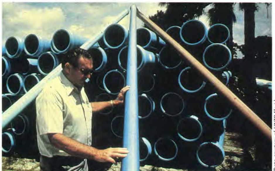
In dual distribution systems, color coding (blue for freshwater, brown for reclaimed water) identifies the nature of the water supply being sent through the pipe.
