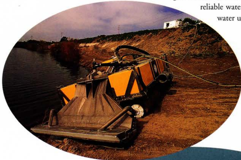
After the Basin Cleaning Vehicle enters a lake, the patented hood will separate sand from silt, returning the sand to the lake bottom and sending the silt to a collection basin via an umbilical hose.
