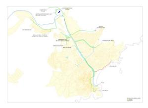
Figure 4. Reclaimed water distribution system of Tossa de Mar in early 2011. Green lines are existing pipeline and red lines are pending infrastructures.
