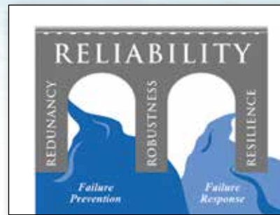
Representation of a reliability framework for direct potable reuse. The two strategies for achieving reliability are failure prevention (through redundancy and robustness) and failure response (through resilience).
